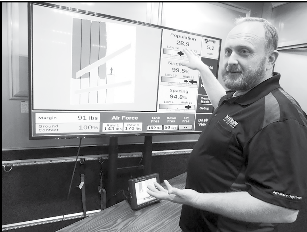
(Courtesy Northeast Community College) Lonny Mitchell demonstrates section control and variable rate technology used for seed placement when planting. Mitchell, who is the precision agriculture trainer at Northeast Community College in Norfolk, is shown with the Precision Agriculture Learning simulator that is used for educational trainings.
